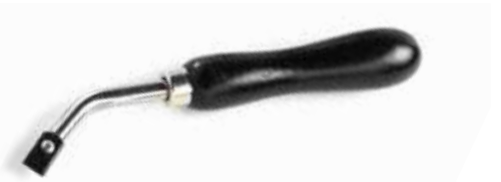
F7110 P Type Grooving Tool This tool cuts a groove in hard or safety flooring prior to welding the flooring sheets together. The replaceable blade on the front is made from sprung steel. F7110B U Shape Grooving Blades x10
